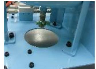
※Like right picture shows , please open this ball valve and leave it open for some time in atmospheric pressure.
