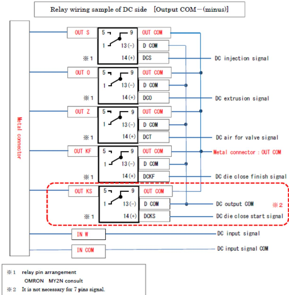
On the occasion of direct output from DC machine, please set independent system and make sure a contact with no voltage.
